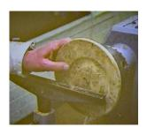
To finish the foot of the bowl and remove evidence of chucking Tom has a board with a piece of carpet stuck onto the surface which he mounts in the chuck. The bowl is sandwiched between the carpet surface and the tailstock. The carpet covered board acts as a friction drive. The foot can then be tidied up.
